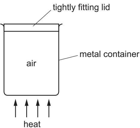
The container is heated strongly behind a safety screen. The lid is blown off by the increased pressure of the air inside the container.
