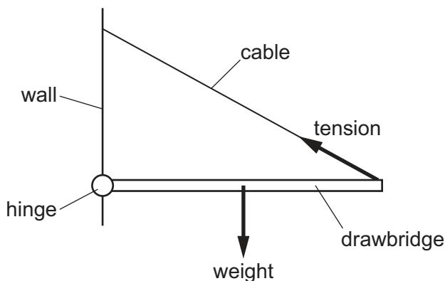
The weight of the drawbridge and the tension in the cable are represented by the labelled arrows in the diagram. There is a third force at the hinge, which is not shown. The drawbridge is in equilibrium.
